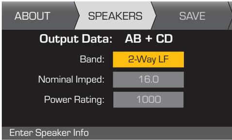
Nominal Impedance and Power Rating are the nominal settings for a single loudspeaker of this type.
