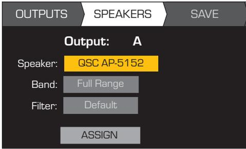
Band and Filter selections are based on the Speaker you select. You must select a loudspeaker before selecting Band and Filter.
